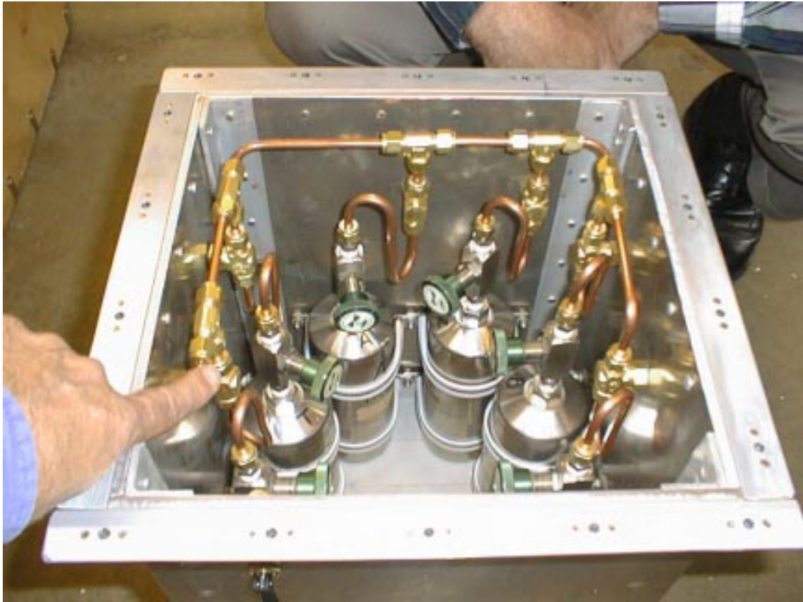
Figure 2-2. Top view of Sampler with Canisters Installed. Left front is attachment point for sample line to CWT.
