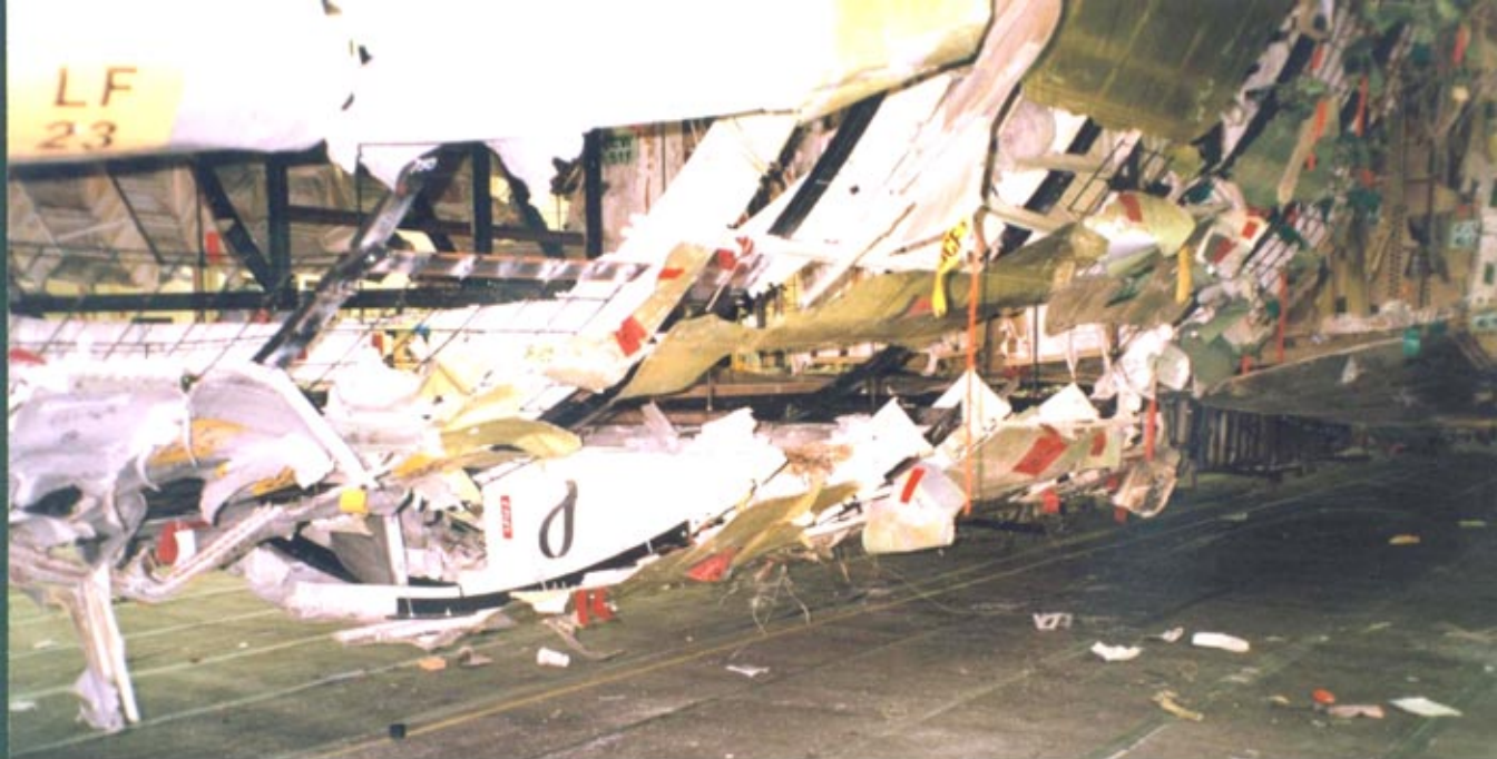
The left side of the red zone crib after it was dropped to match the keel beam from a forward position
