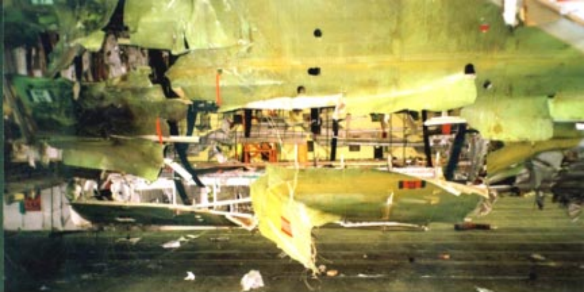
The right side of the red zone crib after it was dropped to match the keel beam from a side position
