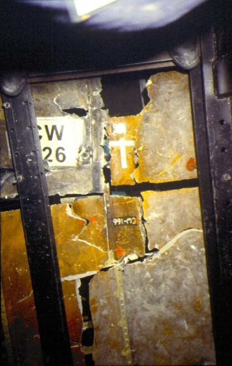
Smaller pieces of the center wing fuel tank including CW166
