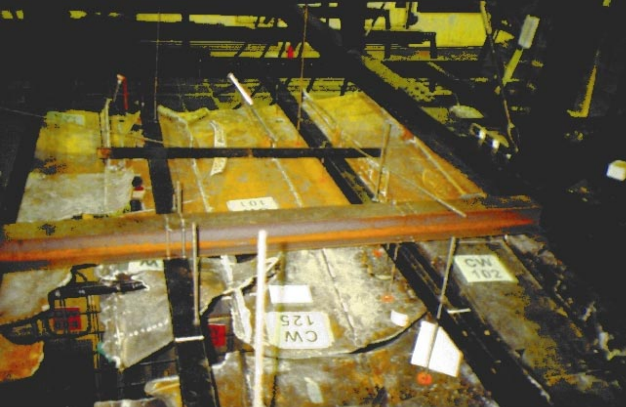
The top of the center wing fuel tank, including CW 125, 102, and 101
