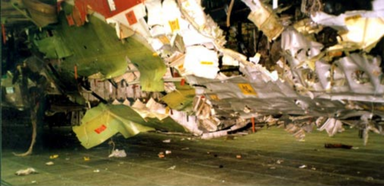
The right side of the red zone crib after it was dropped to match the keel beam from a forward position
