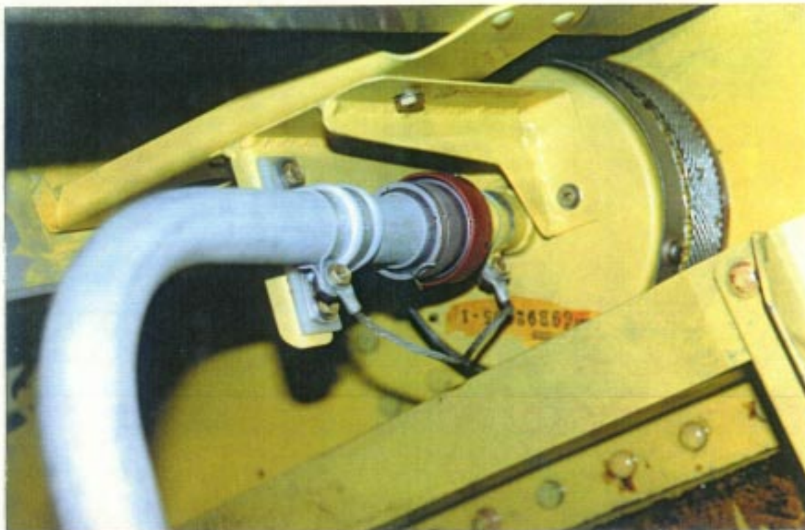
Photo 6: Wiggins couplings (in red) connect fuel tubing in B-747 CWT
