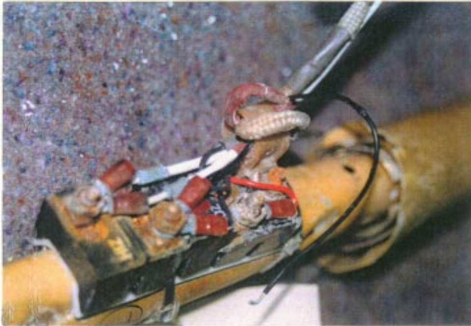
Photo 1: FQIS fragment #36 with large strain relief clamp
