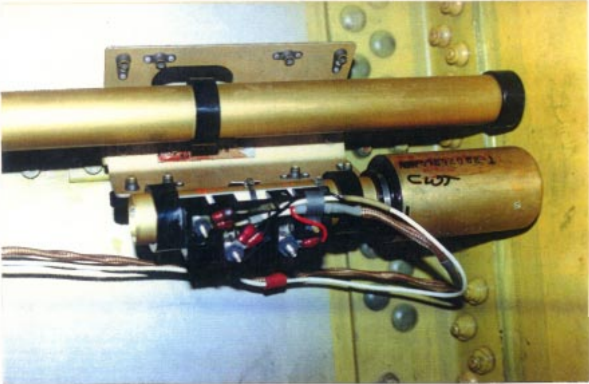
Photo 14. CWT fuel compensator & lower portion of fuel quantity probe
