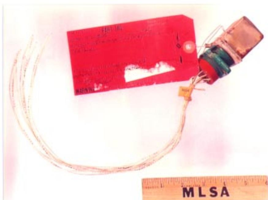
Figure 1. Scavenge pump relay, as received.
