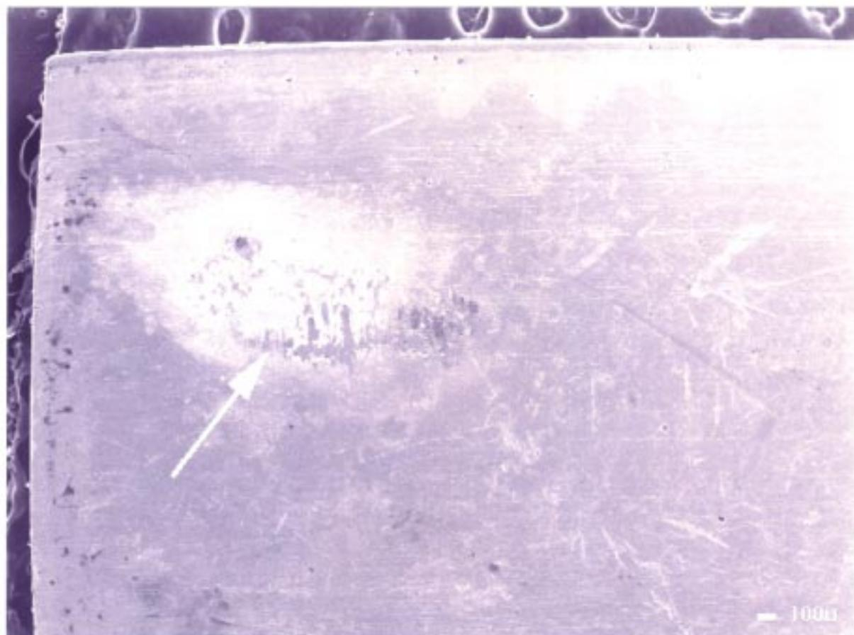
Figure 15. Mating surface of moving contact A2. Arrow shows the contact area.
