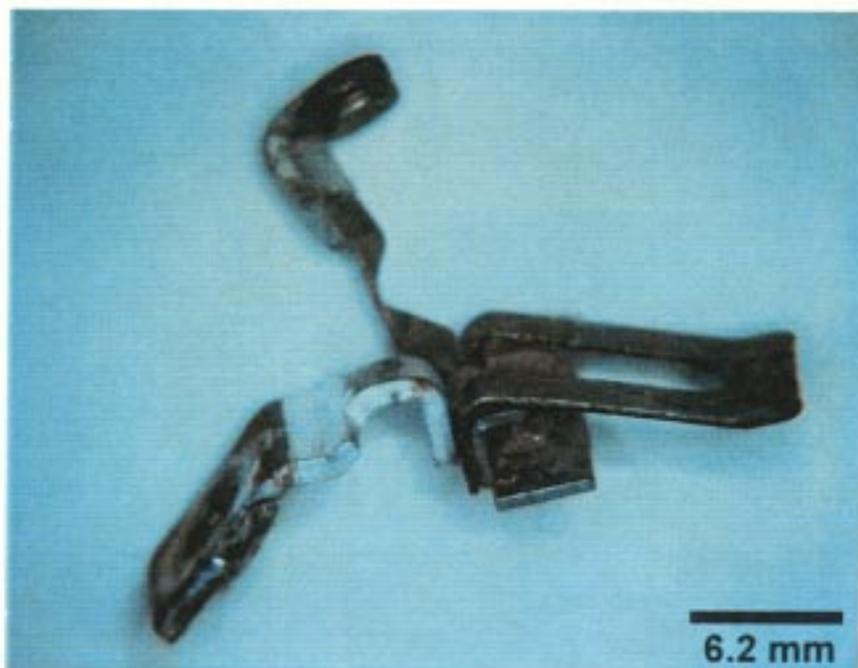
Figure 18. The stationary load terminal and contact of the RTV circuit breaker have a tarnished appearance.
