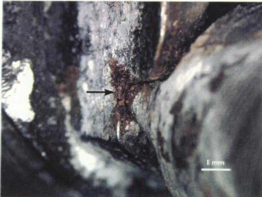
Figure 14. The left side of the scavenge pump switch indicating the knob had been displaced towards the right.
