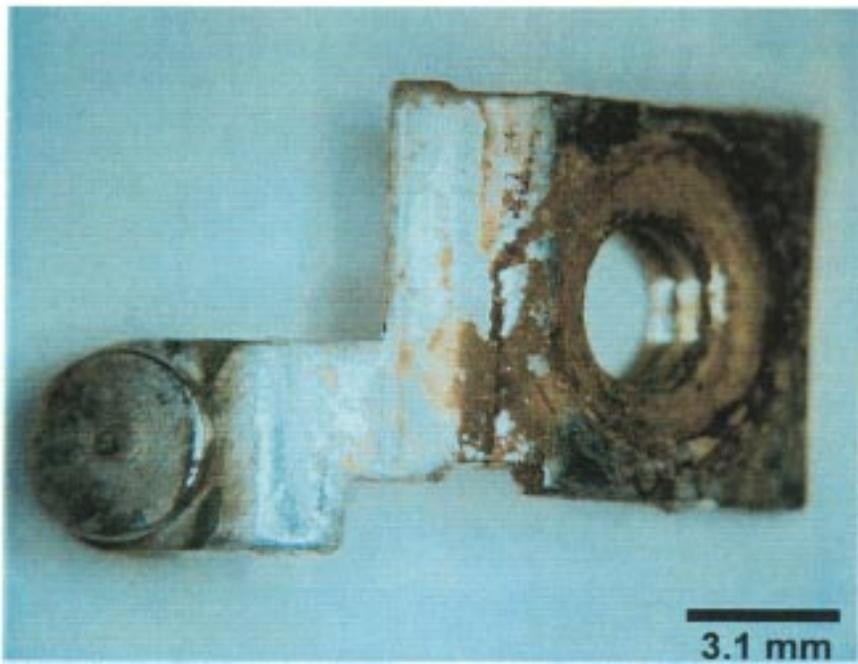
Figure 17. The stationary line terminal and contact of the RTV circuit breaker have a tarnished appearance.
