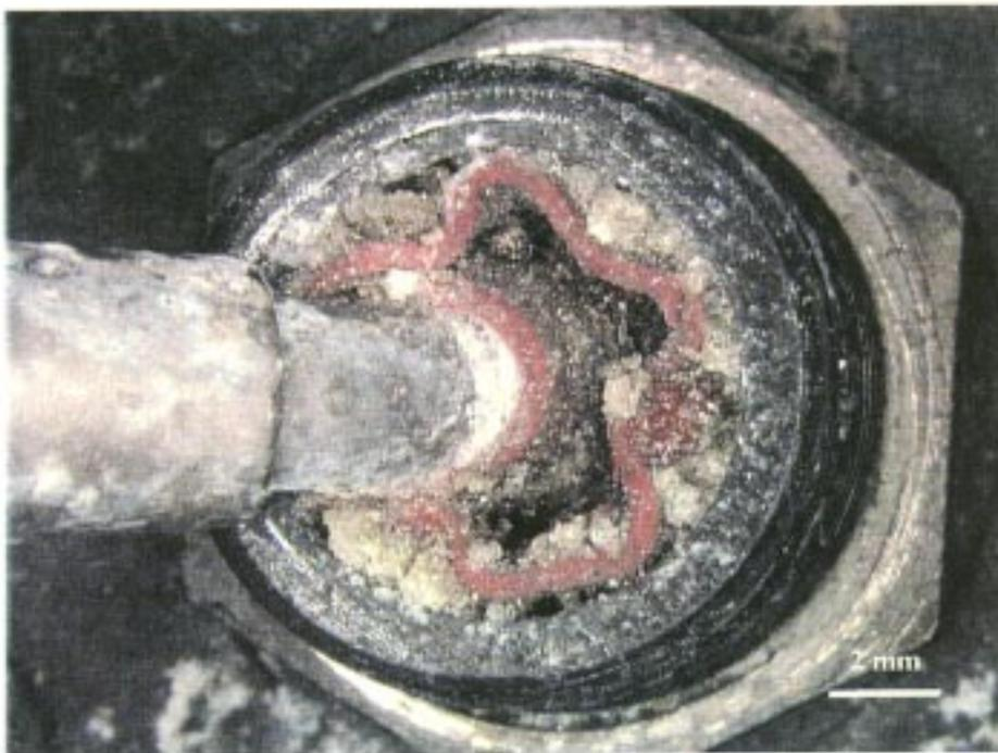
Figure 6. The environmental seal of the left jettison switch exhibiting corrosion and salt water-like deposits.
