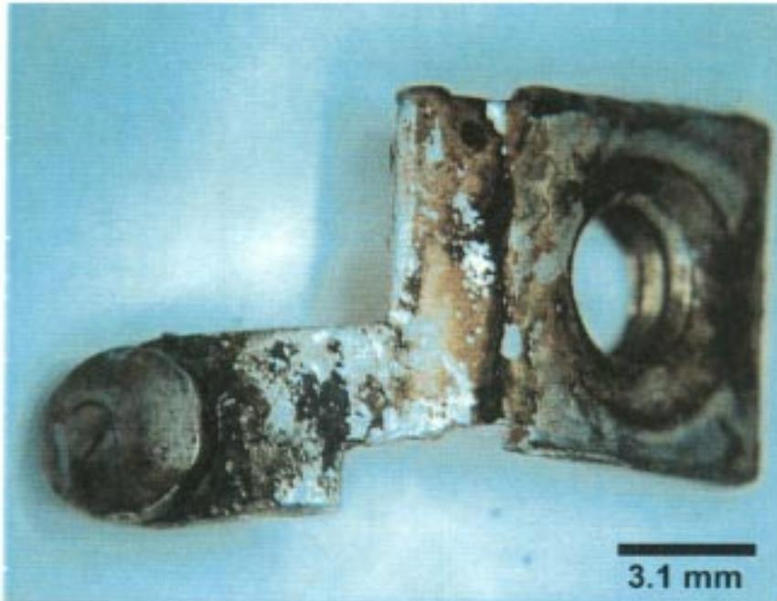
Figure 7. The stationary line terminal and contact of the SPR circuit breaker have a tarnished appearance.
