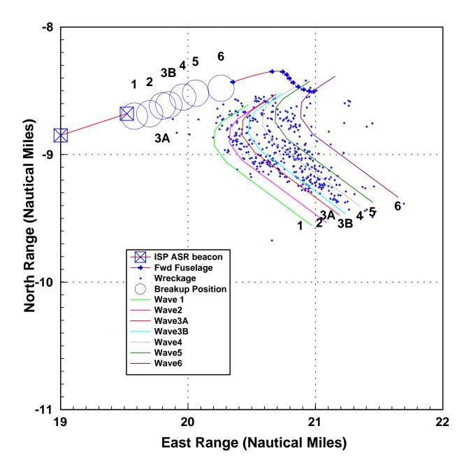
Wreckage Trajectory by Wreckage Band
