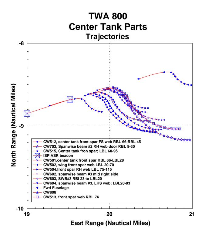
Lower Fuselage Interior (Beneath Center Tank) Trajectories
