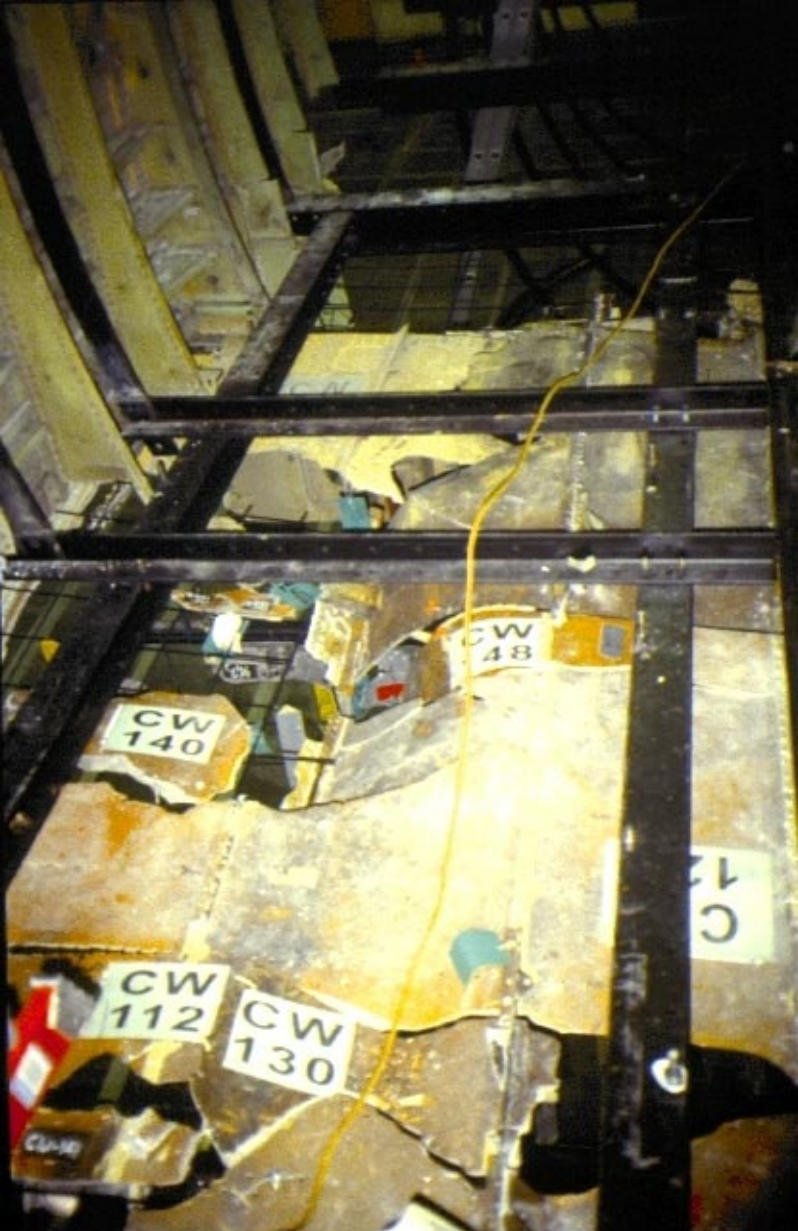
Top of the center wing fuel tank, looking at CW130, 112, 140, 148 and the mesh that was placed to attach smaller pieces
