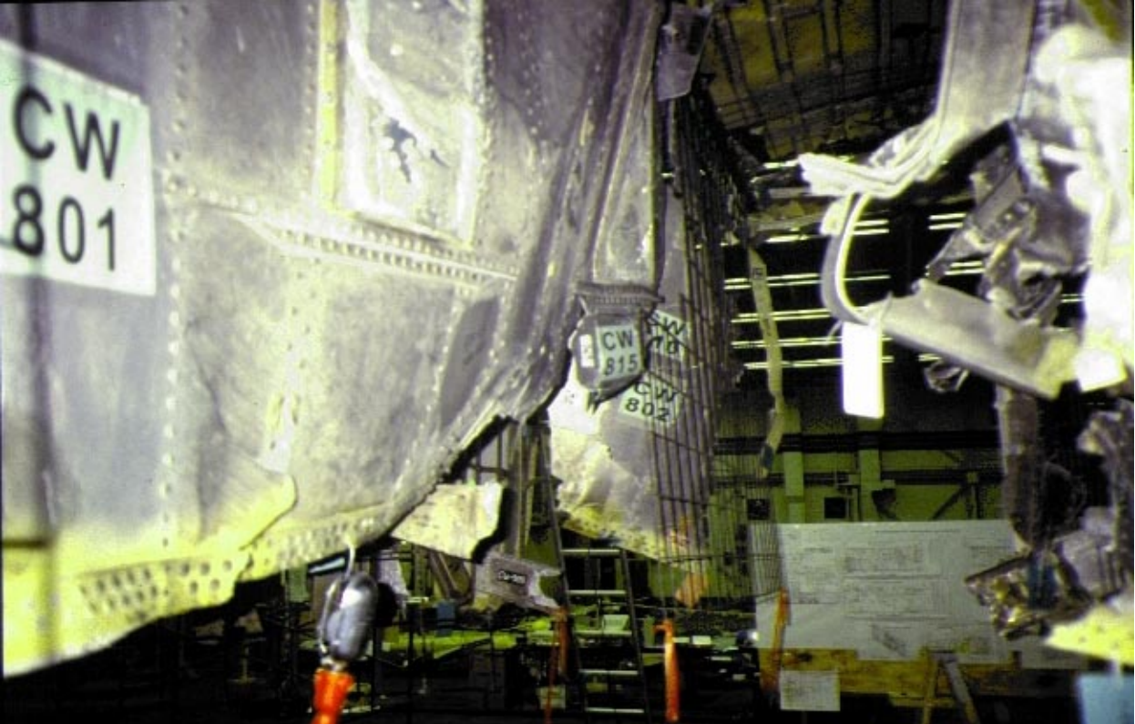
Looking at the mid spar including CW801, 815, and 802 from the right to left side
