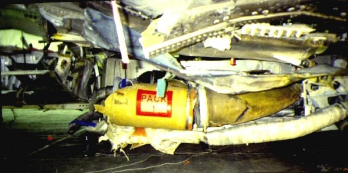
Pack 1 in place
