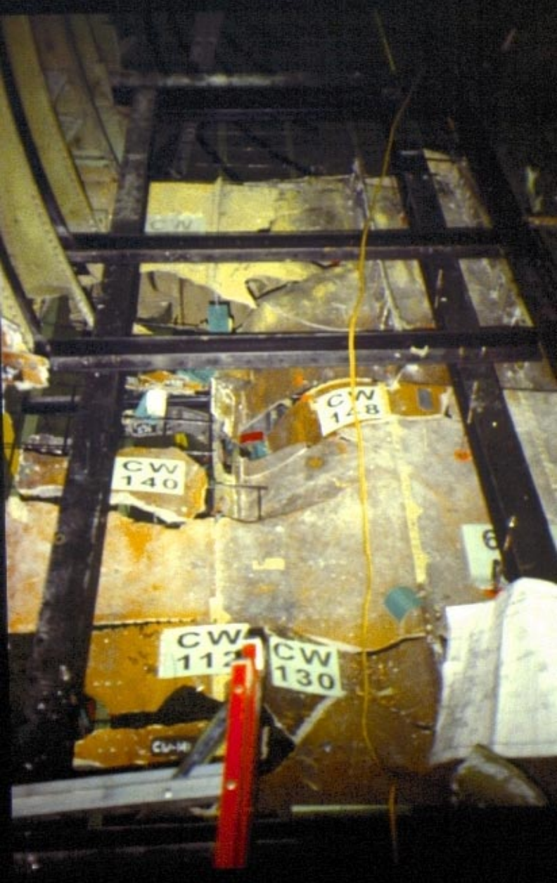
Top of the center wing fuel tank, looking at CW130,112,140, and 148
