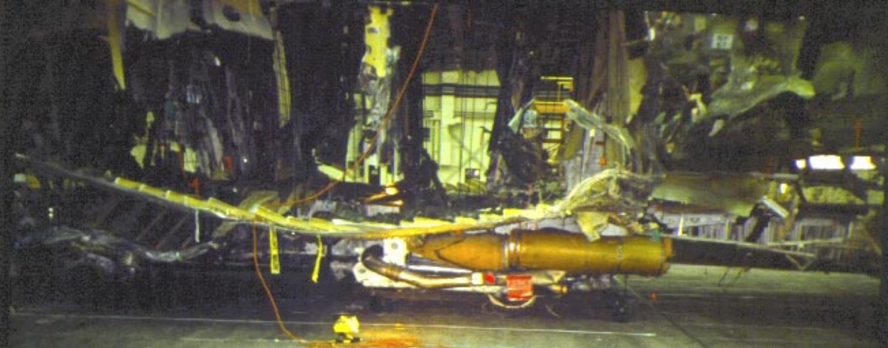
Pack 3 in place under the center fuel tank
