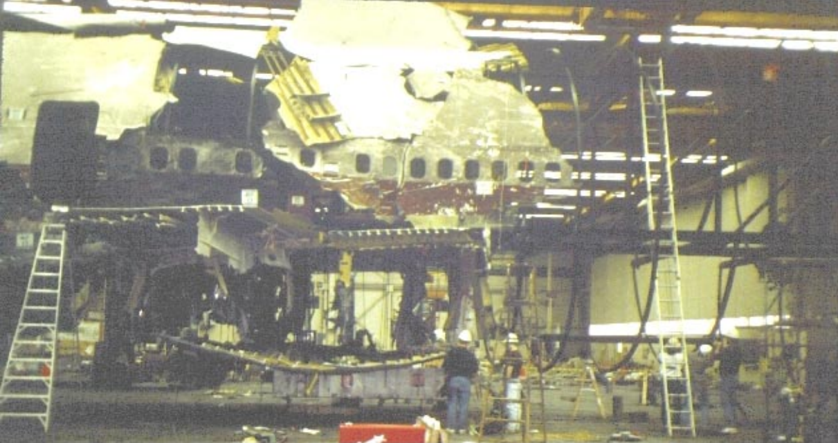
Right side of the center wing fuel tank with bottom floor and portions of the keel beam on March 2
