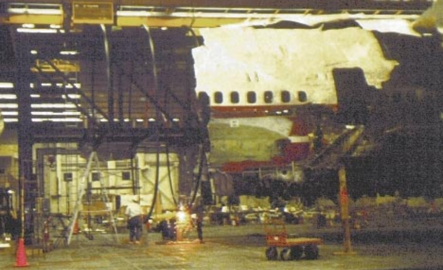
Installing ribs for mesh for the rear cargo area on February 26
