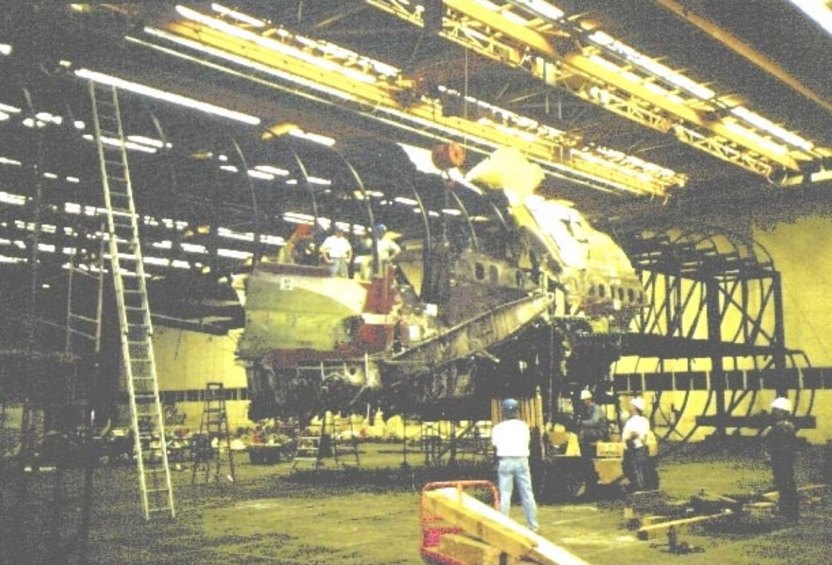
Placing RF38, a large piece with the titanium right side landing gear beam attached on February 18
