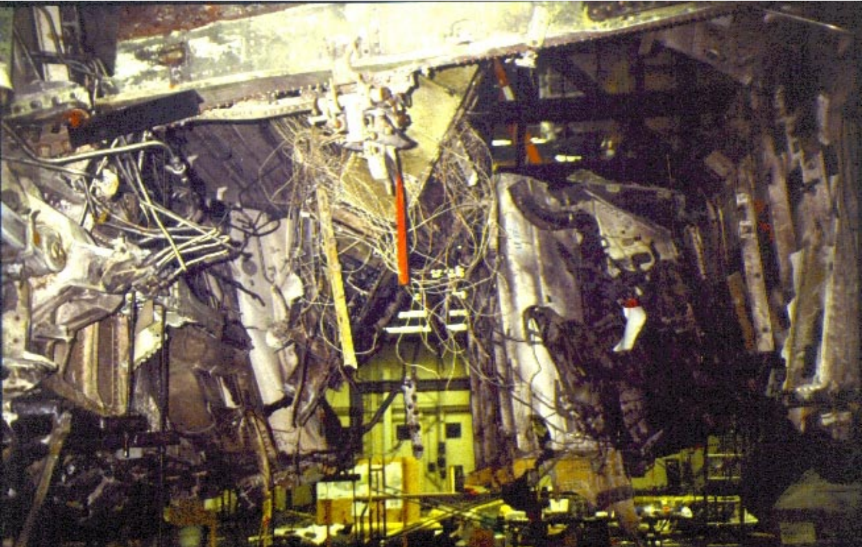
Area of the landing gears, showing pressure deck and the LF40, 0 body line on February 25, looking from right to left
