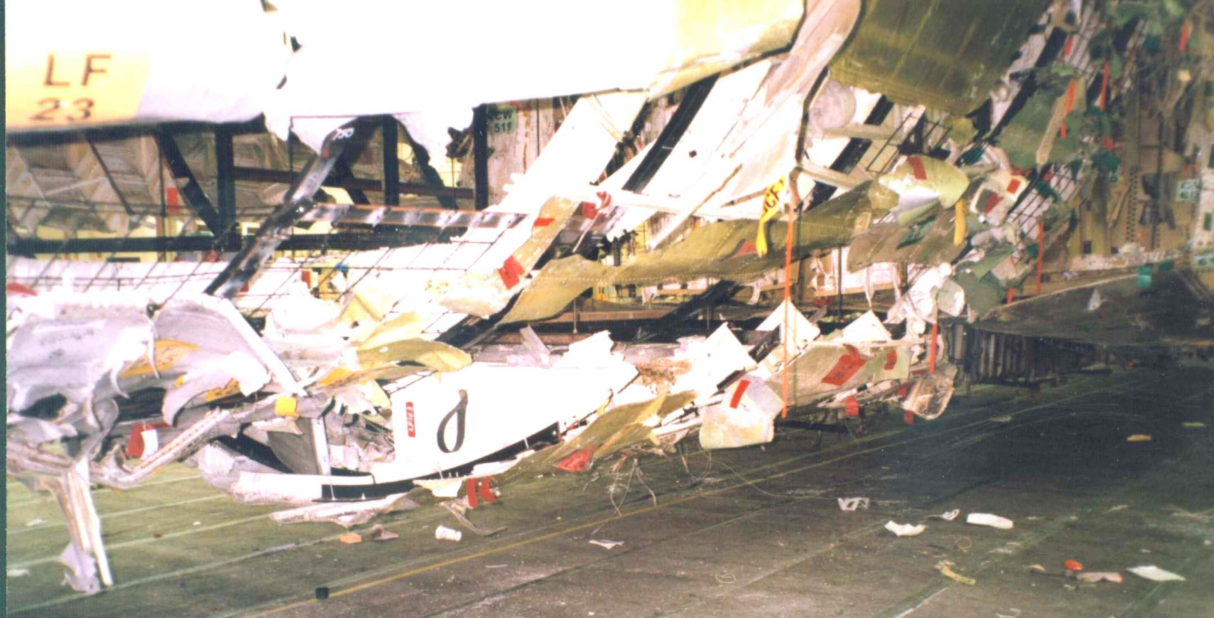
The left side of the red zone crib after it was dropped to match the keel beam from a forward position
