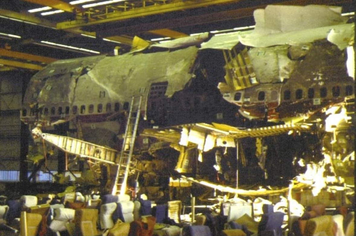
The fuel tank and the left landing gear beam
