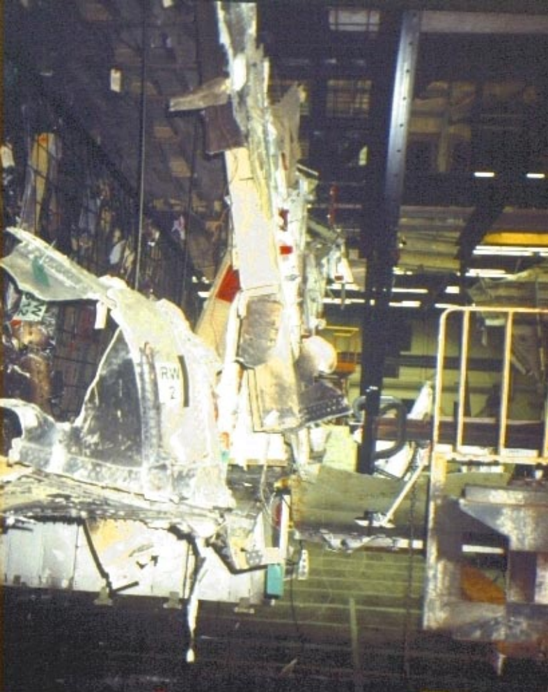
View of RW2, the front spar and the front of the keel beam
